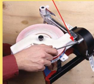
**Quick-Release Tag Guide** opens smoothly with **Slide Block** and provides easy access to tags
